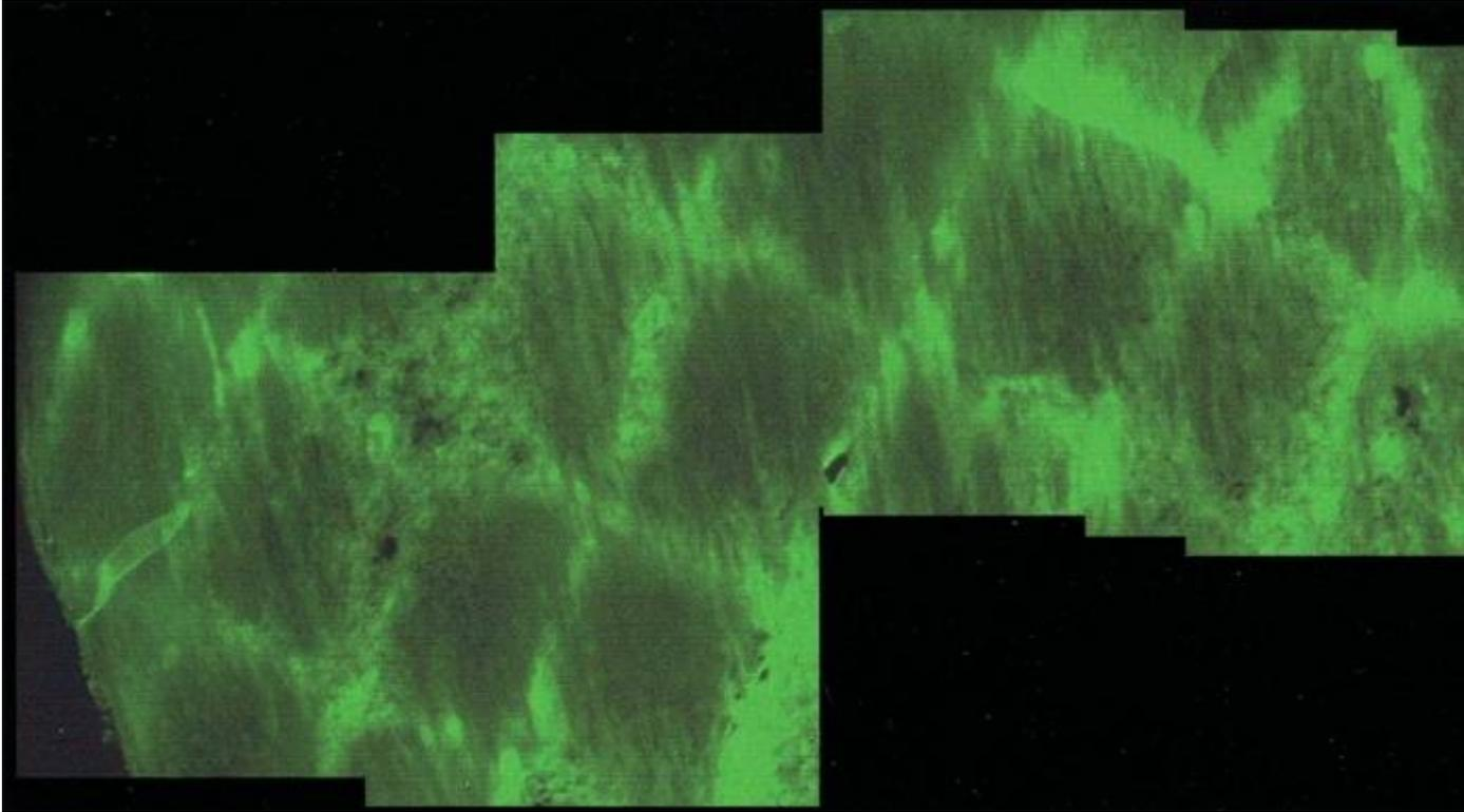
**Scanning Photomicrograph showing inhomogenous drug distribution following stent implantation.**
